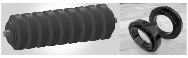
**Conveyor impact roller** is used in loading zone and transfer points applications with excellent absorption ability. It Protects the belt to prevent the lumps, weight or sharp from the free fall of material. The rubber discs are assembled onto an inner heavy-duty steel pipe.
